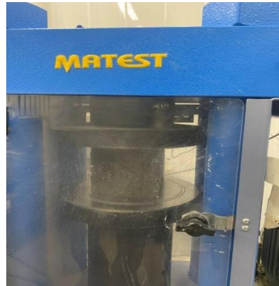
Fig. 1. MATEST Compressive Strength Testing Machine
