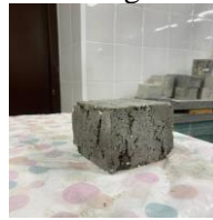
Fig. 7. Crack pattern after loading
