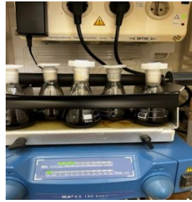
Fig. 1. Adsorption isotherm tests of clay and activated carbon
