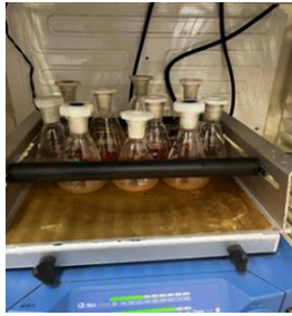
Fig. 1. Adsorption isotherm tests of clay and activated carbon
