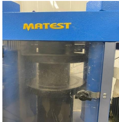
Fig. 1. MATEST Compressive Strength Testing Machine
