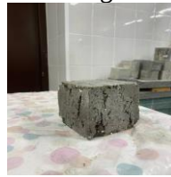
Fig. 7. Crack pattern after loading
