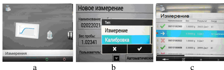
Fig. 3. The sequence of operating modes during calibration of the calorimeter: a – switching to the “Measurement” mode, b – entering the mass of tablets and selecting the operating mode, c – saving the entered data
